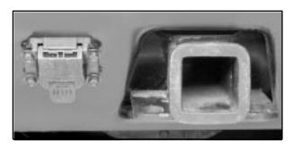
Your vehicle is equipped with the eight-wire trailer towing harness. This harness with a seven-pin universal heavy-duty trailer connector is attached to the rear bumper.
